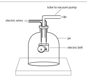
The diagram shows an electric bell inside a jar. The electric bell is switched on and a ringing sound is heard. The air is then pumped out of the jar.
